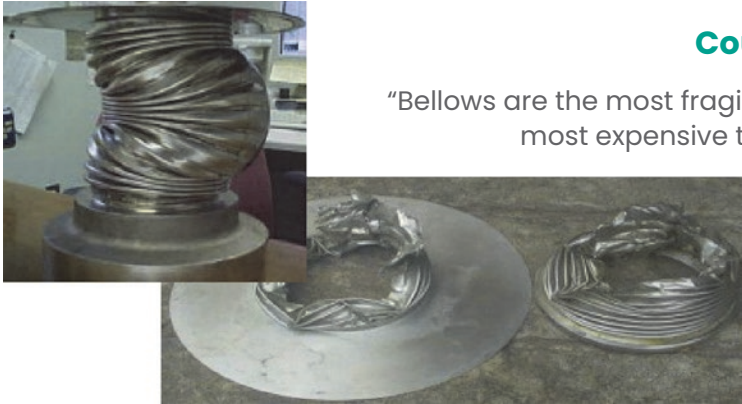
Figure 2 - Damaged bellows from excessive back-pressure and valve chatter
