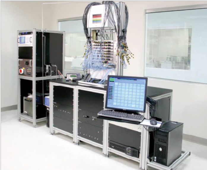
Overall aluminum oxide moisture probe calibration system view
