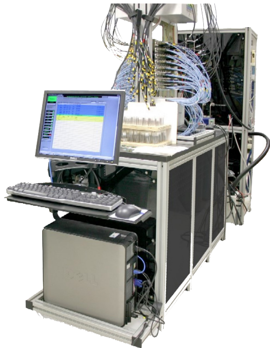
Aluminum oxide moisture probe calibration system
