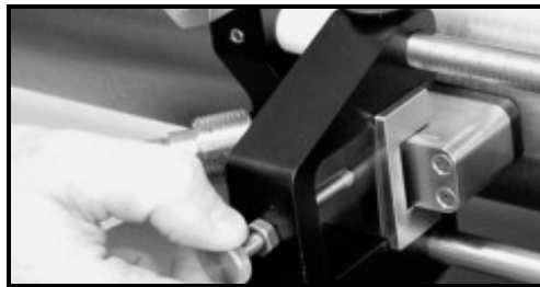
Figure 20: Installing the First Transducer
