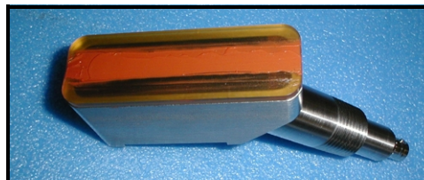
Figure 31: Couplant on Transducer Face
