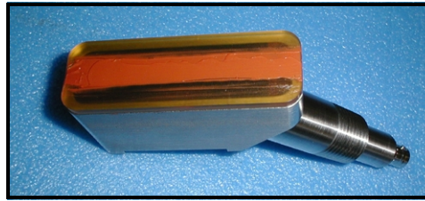
Figure 19: Couplant on Transducer Face
