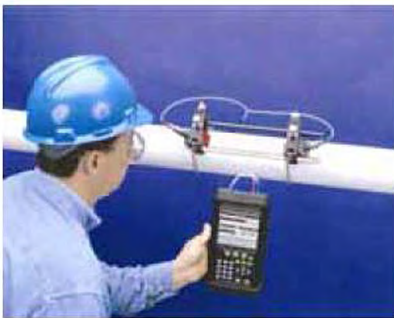
Sample installation of a Panametrics portable ultrasonic flowmeter on a 4" PVC pipe
