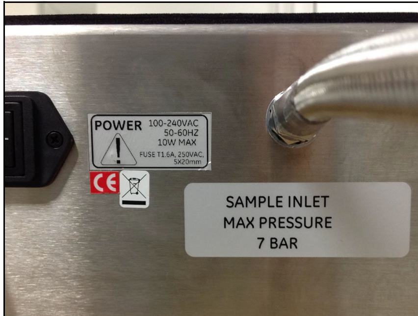
Figure 7: Power, CE and Inlet Labels
