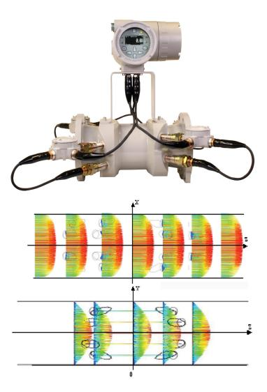
CFD analysis of the ultrasonic port effects. The top graph shows the effect under turbulent flow, the bottom graph under laminar flow conditions. Also not the different flow profiles under these conditions.
