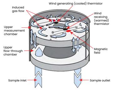
Flow schematic of the XMO2 thermoparamagnetic oxygen measuring cell. Oxygens paramagnetic property causes an oxygen-containing gas sample to move within the magnetic field. The gas movement creates a "magnetic wind" that is sensed by the thermistor pairs. Oxygen concentration and background gas compensation are determined by the transmitters microprocessor.
