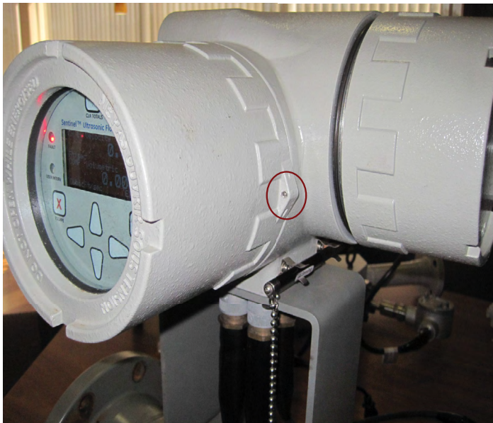
Figure 34: Front cover screwed
