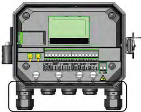
Figure 24: Recommended cable gland usage
