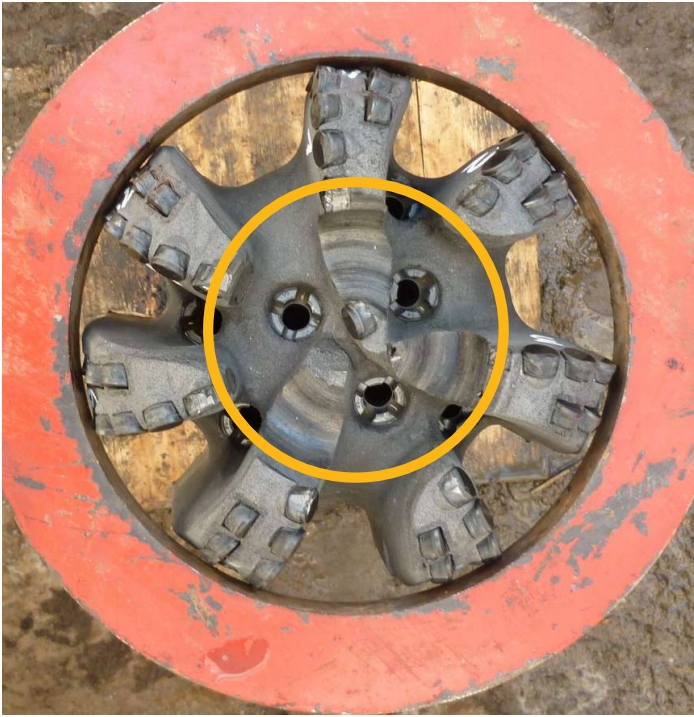
Talon PDC bit with standard chamfer was cored out after drilling 4,272 ft (1,302 m).
