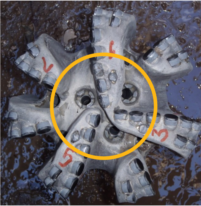
Talon Force bit with StabilisX shaped-cutters drilled 4,983 ft (1,519 m), with minimal damage to the bit.
