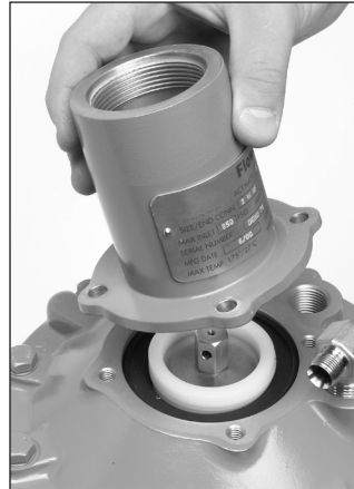
Figure 19 - Removing the spring case
