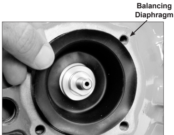
Figure 20 - Replacing the balancing diaphragm
