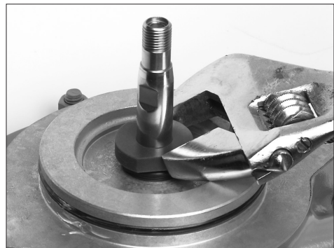
Figure 10 - Removing the stem bushing
