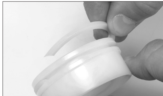
Figure 37 - Installing piston ring on piston
