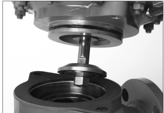
Figure 50 - Remove the actuator housing assembly
