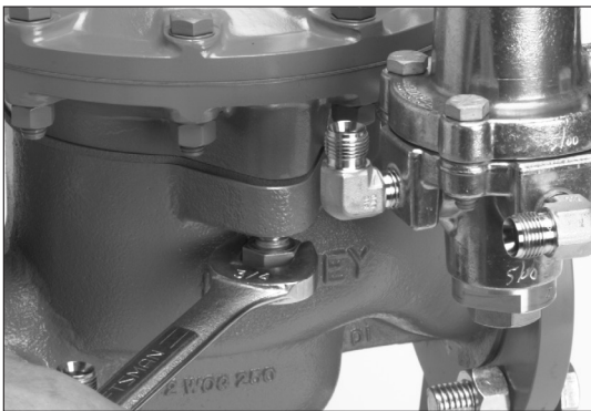
Figure 17 - Tightening the body cap screws
