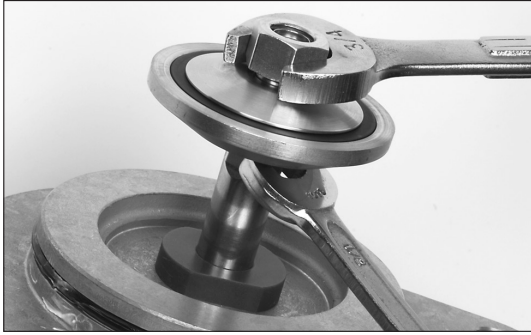
Figure 51 - Remove the stem nut
