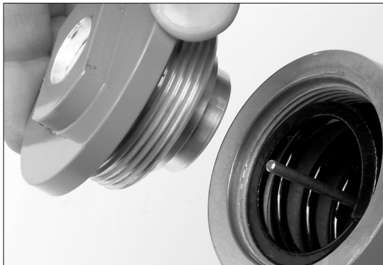
Figure 48 - Installing the spring case cap
