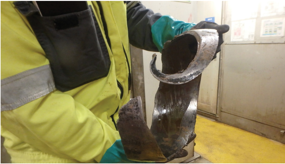
Along with the liner hanger running tool that was stuck in hole at 6,378 ft (1944 m), this piece of aluminum shoetrack was pulled out of the hole by the MASTODON hydraulic pulling tool.
