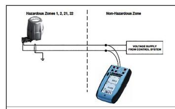
Flameproof instrument may be installed in gas and dust explosive atmosphere of groups IIA, IIB, IIC and IIIC for the zones 1, 2, 21 and 22 with "db" and "tb" protection mode.
