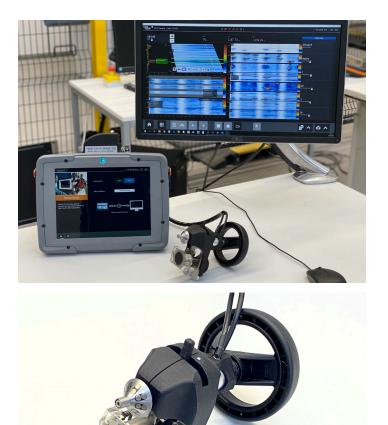
Combining SAMT with our Mentor UT phased array flaw detector's multi-group capabilities lets operators apply defined steering angles and groups to highlight flaws in respect to geometry indications. This capability translates to easier and more informative inspection evaluations.
