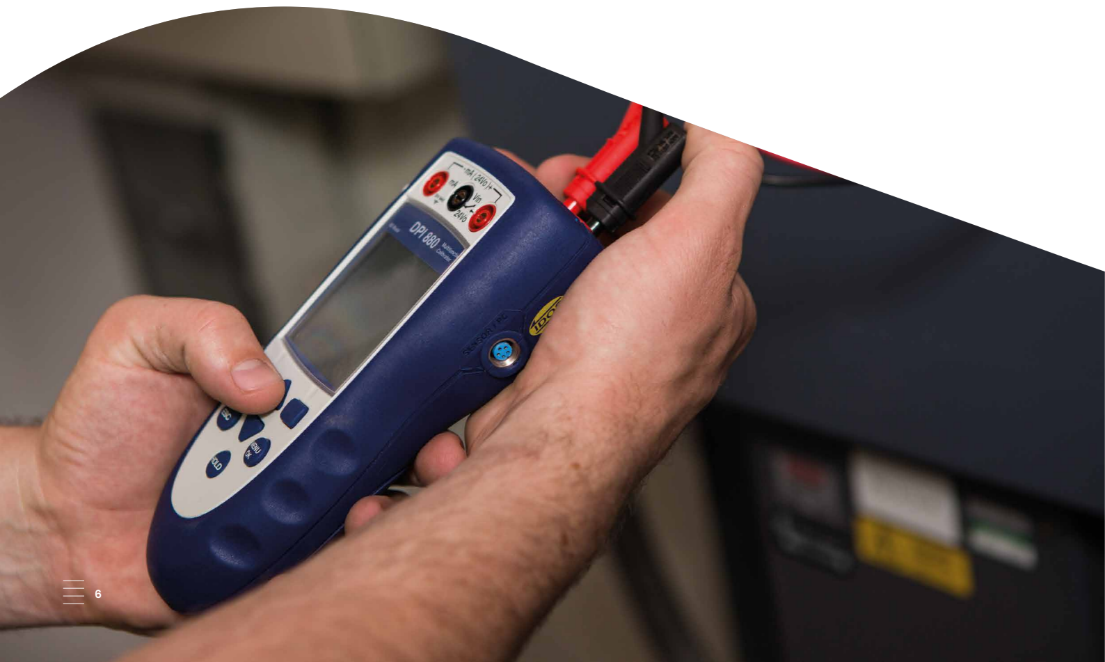
DPI 832 Handheld Electrical Loop Calibrator
