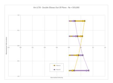
Figure 4. Velocity Profiles Measured by Individual A and B Planes
