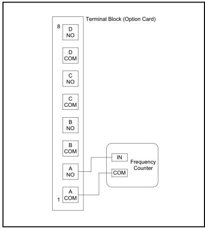
Figure 5: Frequency Counter Connections
