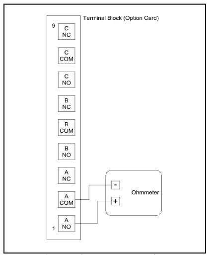
Figure 4: Typical Ohmmeter Connections
