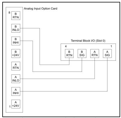
Figure 3: Analog Input Calibration Connections
