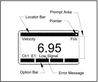
Figure 7: A Typical Display Screen
