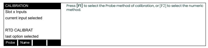
The Probe option allows the meter to calculate the temperature vs. resistance curve, based on input from the RTD in a temperature bath or from an RTD calibrator. The Numer option forces the user to calculate and input the curve values numerically.
