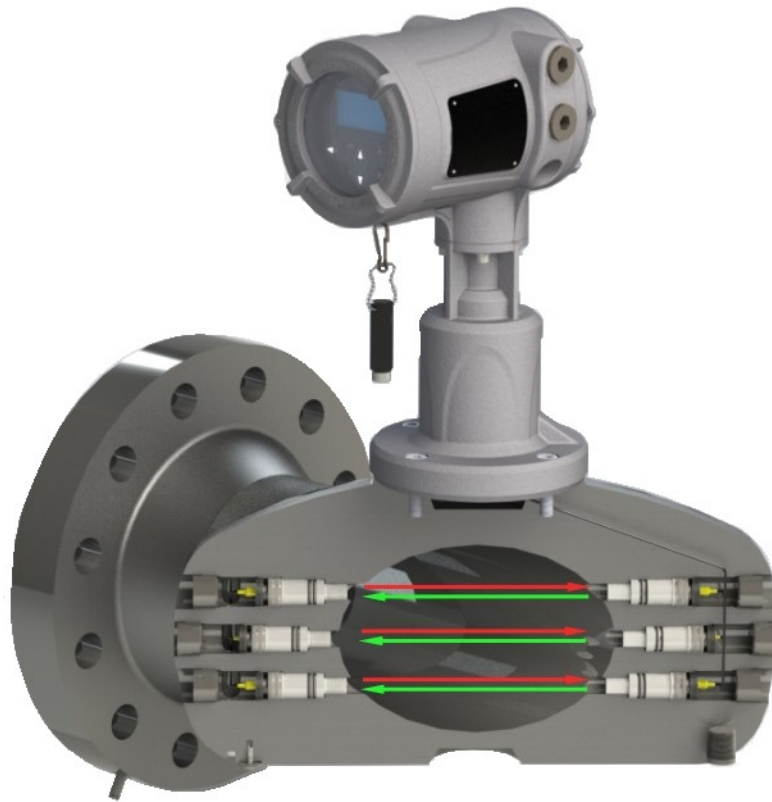
Figure 1: Transducer Paths Across Flow Direction
