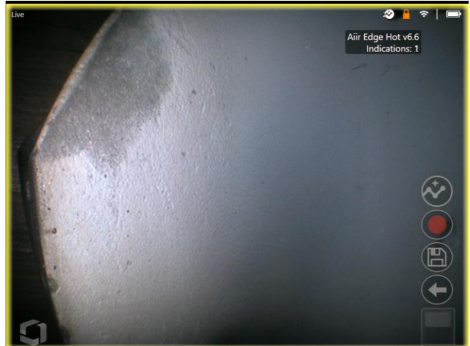
Aiir Edge Hot activated showing the Indication Detected border highlighting presence of defect.
