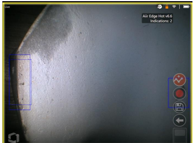
Aiir Edge Hot activated showing the “peek” indication enabled to temporarily visualize the defect location.
