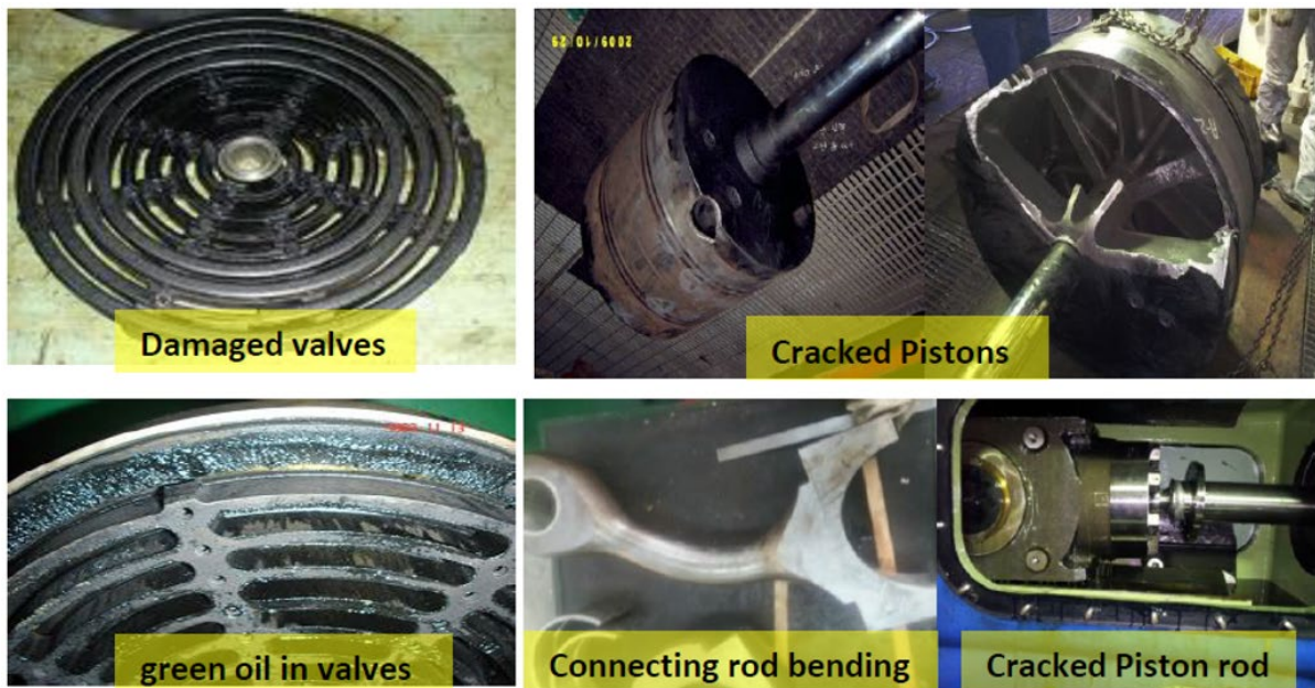
Figure 4. Damaged parts on 3 booster gas compressor
