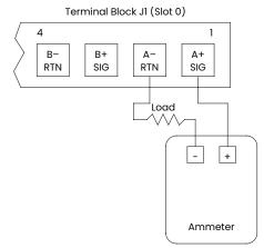
Figure 11: Ammeter connection (output A)
