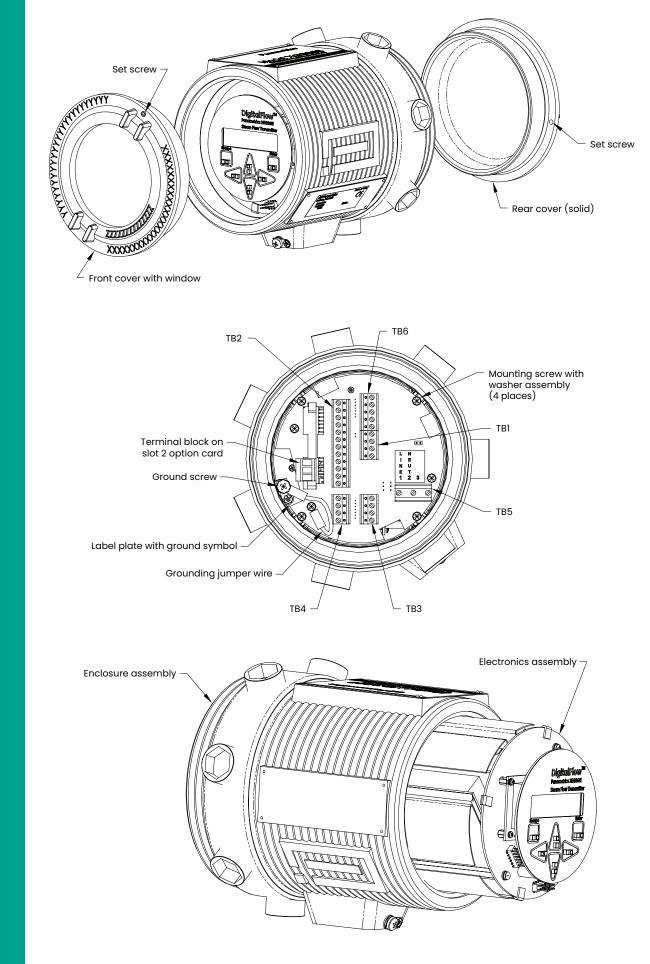
Figure 6: Model XGF868i electronics console assembly
