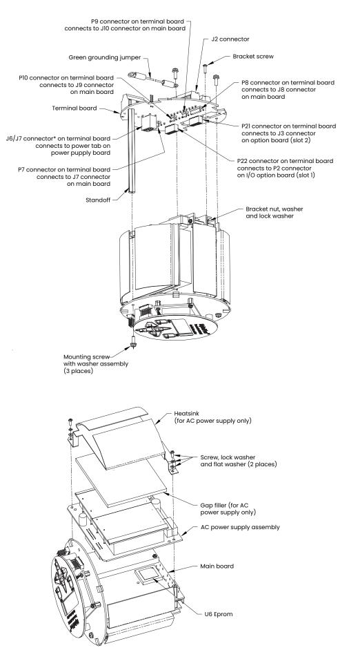
Illustration 8 (shown with AC power supply) Note: There are noheat sink and gap fillers with a DC power supply.
