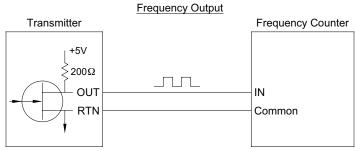
Figure 2: Totalizer and frequency output wiring
