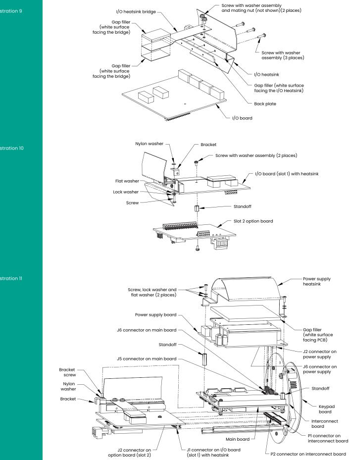
Figure 8: Model XGF868i I/O option card subassembly
