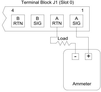
Figure I: Ammeter connection (output A)
