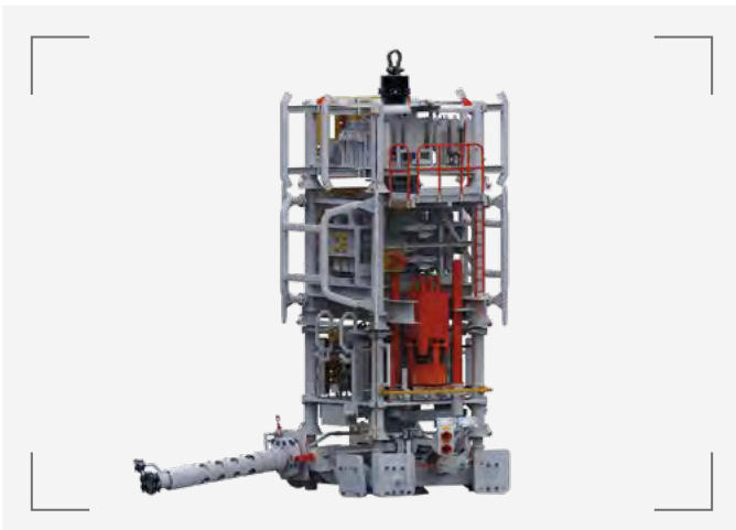
Stack-up sketches of the EDP, LRP, XT, flowbase with flowline connector, tree mounted UTA. Tree is shown with the Modpod SCM installed on an adaptor plate to provide full interchangeability with legacy equipment subsea.
