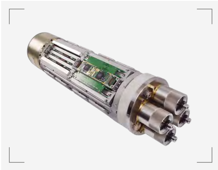
Subsea Electronics Module – SemStar5
