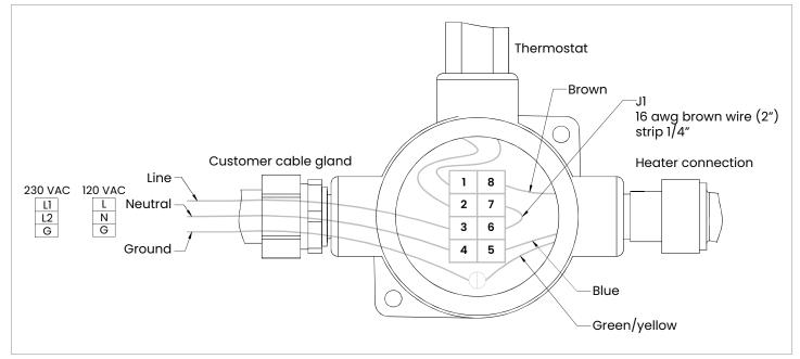
Figure 5: USA/CAN heater wiring diagram
