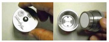
Figure 94: Removing the filter cap
