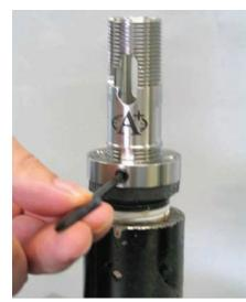
Figure 14: Aligning and tightening the Allen screw
