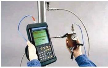
Figure 99: PM880 portable hygrometer
