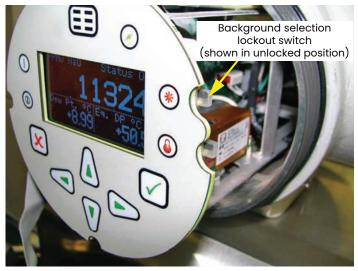
Figure 101: Background selection lockout switch location
