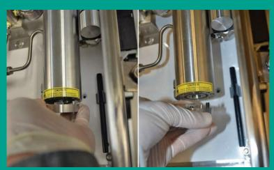
Figure 86: Reinstalling the mirror end cap assembly
