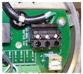
Figure 26: Power terminal block
