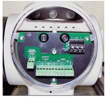
Figure 25: Wiring terminal blocks
