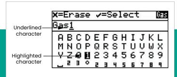
Figure 44: Alphanumeric menu with keyboard highlighted
