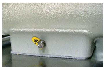
Figure 30: Earth ground connection
