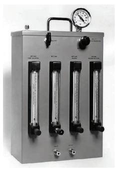
Figure 100: MG101 moisture generator
