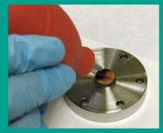
Figure 82: Blowing air onto the mirror
