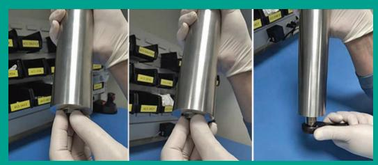
Figure 92: Replacing mirror end cap assembly into the absorption cell
