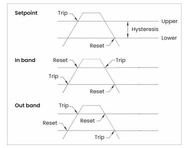
Figure 41: Example of alarm types
