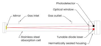
Figure 1: Laser absorption cell, basic elements
