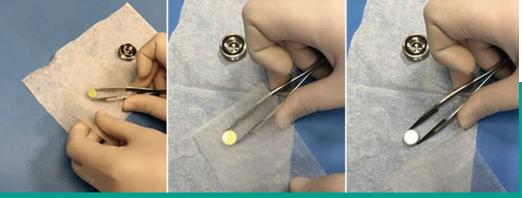
Figure 90: Cleaning a contaminated mirror
