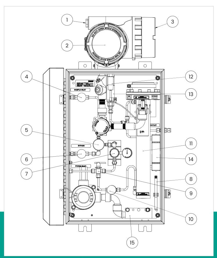
Figure 2: Aurora H2O system assembly with optional USA/CAN heater
