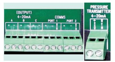
Figure 28: (Left)Input/output connections Figure 29: (Right) Pressure transmitter connections
