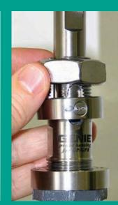
Figure 21: Loosening the insertion nut
