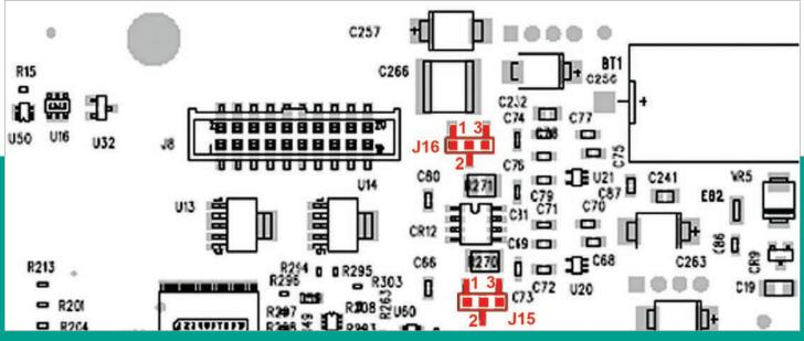
Figure 27: RS-485 mode termination - install jumpers at J15 and J16, pins 1 and 2
