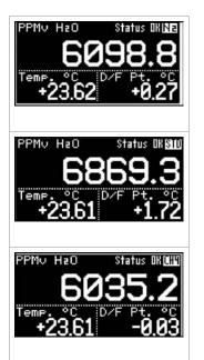
The **Aurora H2O** displays the selected background gas an indicator in the upper right corner of the LCD, adjacent to the status message. Gas Data Background Gas Mol. Wt. Z Factor Label From the gas data menu, select background and press enter. The following screen appears.
