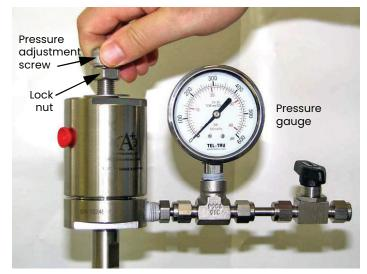
Figure 23: Turning the pressure adjustment screw
