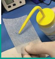
Figure 89: Applying acetone to lens tissue
