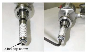
Figure 16: Checking/tightening the Allen cap screw
