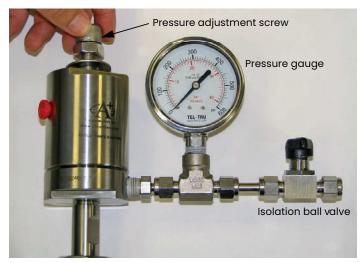
Figure 17: Rotating the pressure adjustment screw
