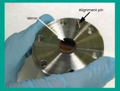
Figure 80: Handling the mirror assembly
