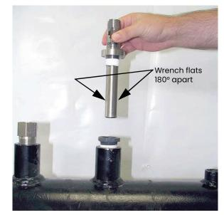
Figure 13: Tightening the housing
