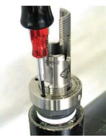
Figure 15: Tightening the Allen screws
