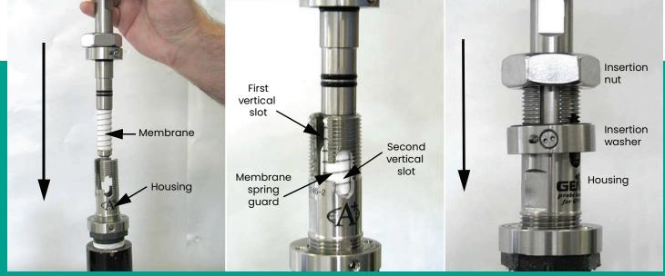
Figure 18: Installing the probe
