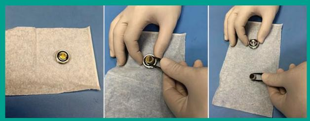
Figure 88: Inspecting the mirror assembly
