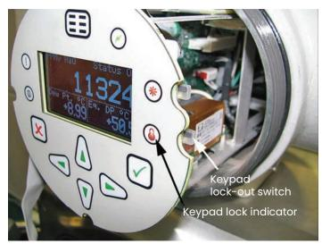
Figure 37: Keypad lock-out switch location
