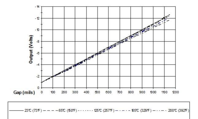
Figure 4: Typical 3300 XL 50 mm Probe + 1m Cable @ High Temperature (Proximitor Sensor + 8m of Extension Cable @ 25 °C)
