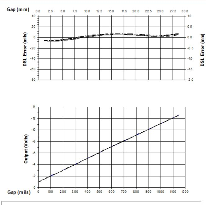
Figure 6: Typical 3300 XL 50 mm 5 m Proximitor Sensor with 4 m Extension Cable @ High Temperature (Probe is at 25°C)
