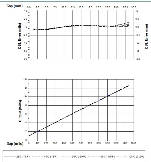
Figure 8: Typical 3300 XL 50 mm 9 m Proximitor with 8 m of Extension Cable @ High Temperature (Probe is at 25°C.)
