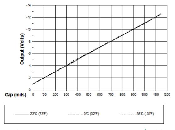
Figure 3: Typical 3300 XL 50 mm Probe + 1m Cable @ Low Temperature (Proximitor Sensor + 8m of Extension Cable @ 25 °C)
