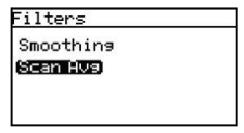
The Scan Average setting is used to change system noise rejection. By averaging entire scans, the Signal/Noise Ratio (SNR) can be increased. This is particularly useful in the presence of certain background gases, which can interfere with the moisture absorption peak, or introduce background noise.
