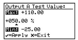
**Note:** The output value will change immediately, it is not necessary to select Apply.
