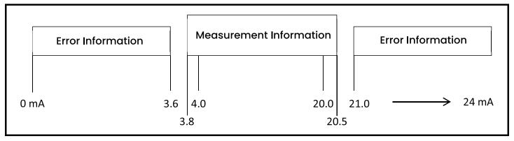
Figure 9: NAMUR output value ranges
