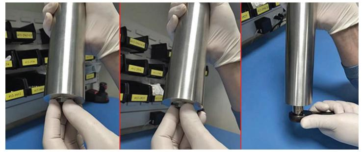
Figure 59: Replacing mirror end cap assembly into the absorption cell
