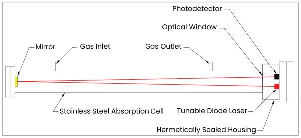
Figure 1: Laser absorption cell, basic elements
