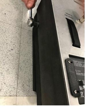
Figure 53: Extraction of absorption cell end mirror from inner foam housing while holding the assembly upright to prevent the mirror from falling out
