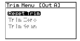
Use the left or right arrow keys to highlight YES and press **Enter**. This cancels any previous trim values, and returns the **Aurora TransPort** to its factory adjustment. The display returns to the previous screen with Trim Zero highlighted.
