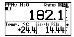
After startup, the screen will need to be unlocked. To unlock the screen, select [x] Cancel,  $[\sqrt{}]$  Enter, [x] Cancel in sequence.
