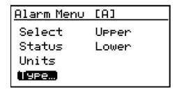
Use the arrow keys to select an alarm type. Press **Enter** to save (or **Cancel** to keep the previous value), and return to the Alarm Menu.
