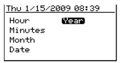
Use the left and right arrow keys to select each digit to be changed. Use the up and down arrow keys to change the value. When finished, press **Enter**. The screen returns to the Clock Menu.
