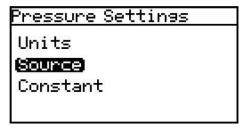
Use the left and right arrow keys to select the line pressure source. Live accepts a pressure value from a pressure transmitter and **Remote** accepts a value via a Modbus connection. To set a constant value, select Constant and press **Enter**. The screen returns to the Pressure Menu.
