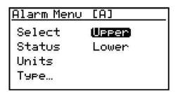
Use the left and right arrow keys to select each digit to be changed and the up and down arrow keys to increase or decrease its value. Press **Enter** to save (or **Cancel** to keep the previous value), and return to Alarm Menu.
