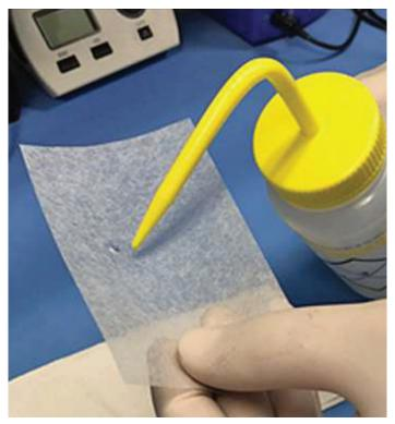
Figure 56: Applying acetone to lens tissue
