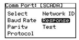
Use the left and right arrow keys to select each digit to be changed. Use the up and down arrow keys to change the value. When finished, press **Enter**. The screen returns to the Comm Port Menu. A value of zero permits the Aurora to respond immediately. Do not specify a response delay longer than absolutely necessary, as this limits message throughput.
