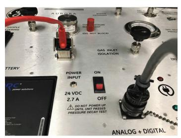
Figure 3: Aurora TransPort 1/0 cable connections
