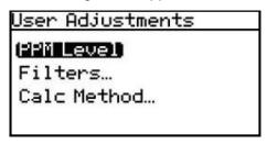
Use the left and right arrow keys to select each digit to be changed. Use the up and down arrow keys to change the value. When finished, press **Enter**. The screen returns to the User Adjustments Menu.
