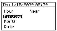
Use the left and right arrow keys to select each digit to be changed. Use the up and down arrow keys to change the value. When finished, press **Enter**. The screen returns to the Clock Menu.
