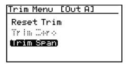
This will cause the Aurora TransPort to output 20.000 mA on the output being trimmed. The output value should then be read using the connected recorder, SCADA equipment, or DVM. Enter the value read from the connected equipment as the Span Trim value.
