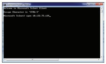
Figure 75: Telnet OPEN command
