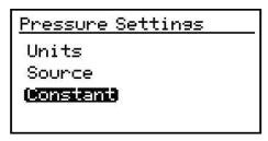
Use the left and right arrow keys to select each digit to be changed. Use the up and down arrow keys to change the value. When finished, press **Enter**. The screen returns to the Pressure Menu.
