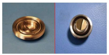
Figure 58: Replacing cleaned mirror into end cap assembly
