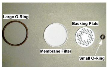
Figure 66: O-Rings, membrane filter and backing plate removed
