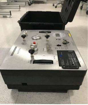
Figure 52: Extraction of inner foam assembly from TransPort Pelican case for access to absorption cell end mirror
