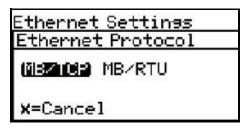
To use Modbus/TCP over Ethernet, the Ethernet module must also be configured as follows:
