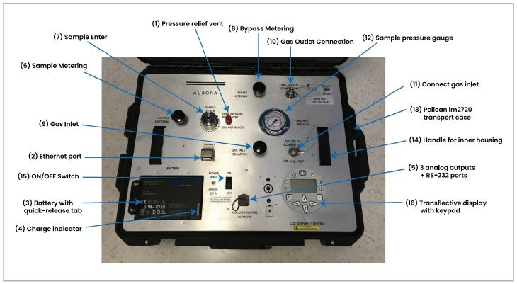
Figure 4: Front panel of BHGE Aurora TransPort
