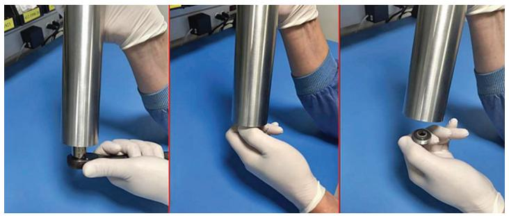
Figure 54: Removing mirror end cap assembly from the absorption cell
