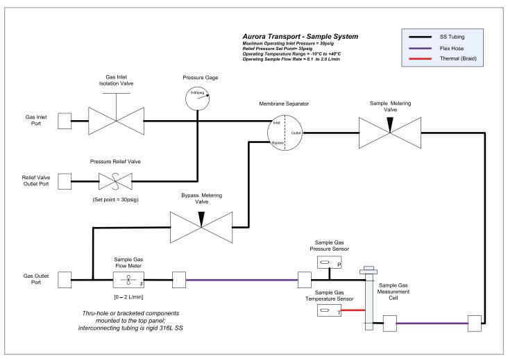
Figure 2: Aurora TransPort integral gas sample system schematic
