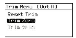
Use the left and right arrow keys to select each digit to be changed, and the up and down arrow keys to increase or decrease its value. Press **Enter** to save (or **Cancel** to keep the previous value).
