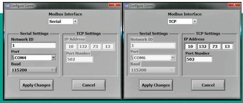
Figure 39: Serial (Left) and TCP (Right) screens
