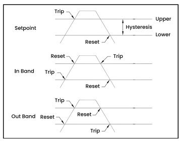
Figure 10: Example of alarm types
