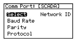
To select a communication port, use the arrow keys to highlight Select and press **Enter**. The following screen appears.
