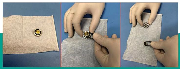
Figure 55: Inspecting the mirror assembly
