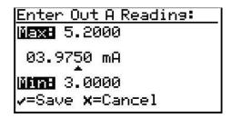
The Trim Menu returns with Trim Span highlighted. To change the span value, press Enter. A screen similar to the following appears.
