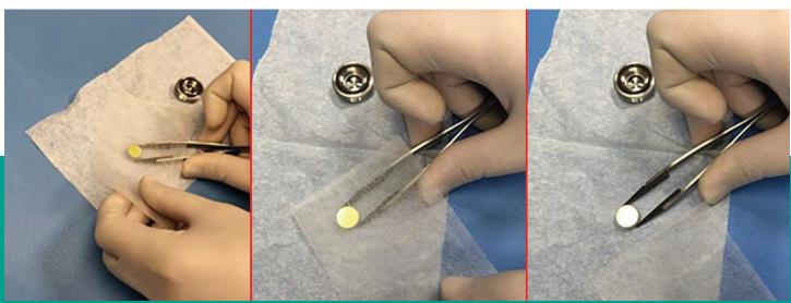
Figure 57: Cleaning a contaminated mirror
