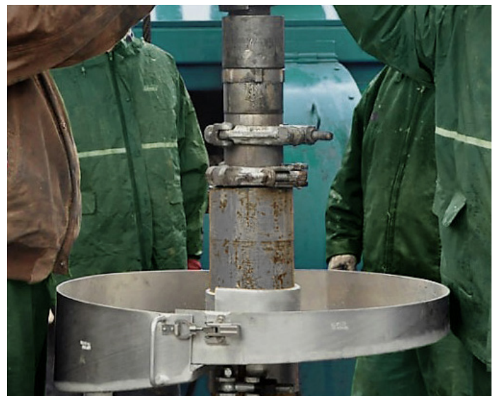
Core recovery: Pollution catch pan
