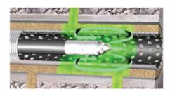
When the plug is soluble, the cleaning action of the gravel pack ensures that fluid moves into the pack where solvent action can occur. Fresh, reactive chemical is delivered, and the spent fluid is displaced as the dissolving action proceeds. A final pass of the Roto-Jet tool flushes residual chemical and reaction products from the pack. Testing indicates when complete flushing is achieved.
